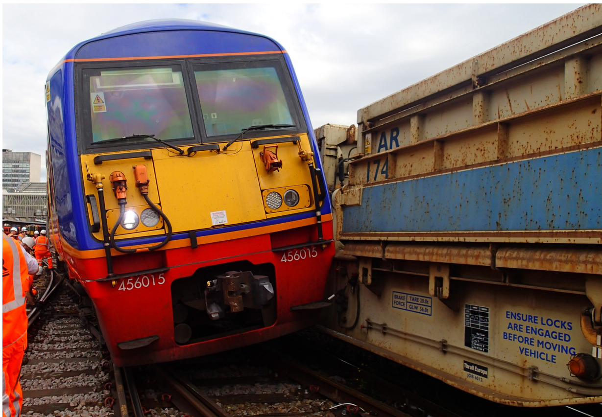
Figure 1: Passenger and engineering trains after the collision
