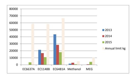
**Note** EC1148B and EC6637A Corrosion Inhibitors, EC6481A hydrate inhibitor and methanol are chemicals used for the wet gas operation and are received at the Terminal for disposal and therefore not discharged to sea
