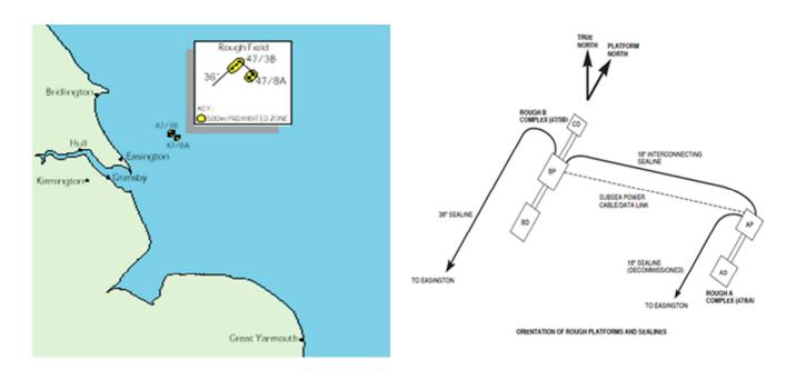
There are two platforms within the Rough Field, Rough 47/8 Alpha and 47/3 Bravo. The Alpha platform comprises two bridge-linked platforms, whilst the larger Bravo platform comprises three bridge-linked platforms. The platforms are approximately 2 kilometres apart and are designed to produce or inject gas via the reservoirs 30 wells.
