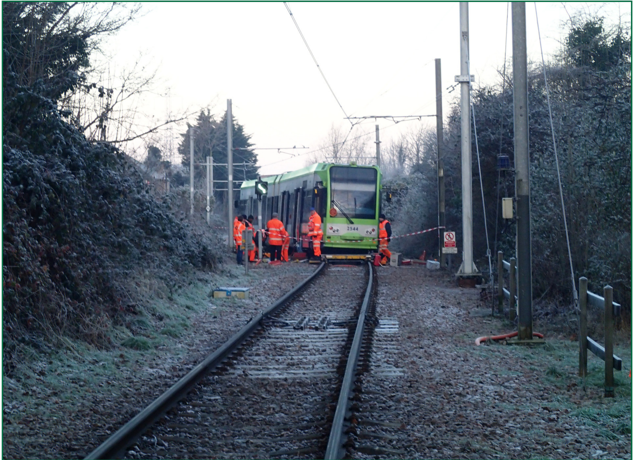
Figure 4: The tram following the derailment, showing the PPI indicating that points MTJ09G are detected for the correct (left) route
