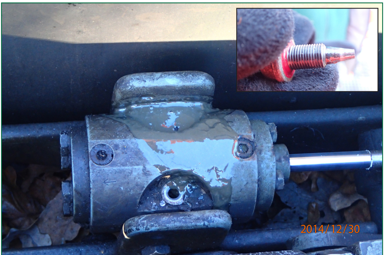
Figure 5: Damper after removal of bleed screws, showing contaminated fluid. Inset: bleed screw, with small particles of grit on the coned end
