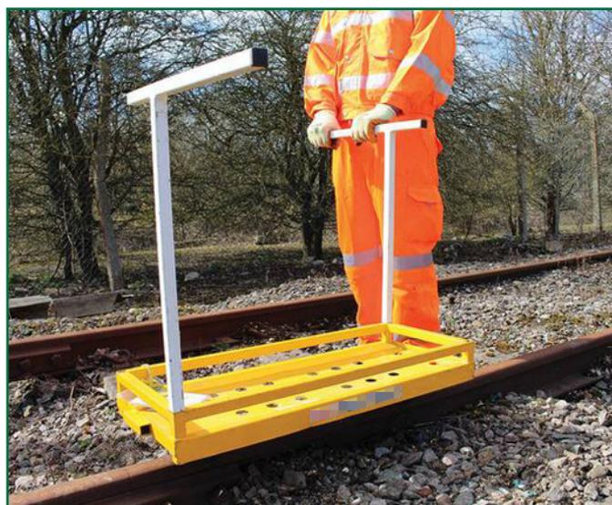
Figure 7: Typical rail skate (not identical to the rail skate used by the workgroup on 27 December 2014)
