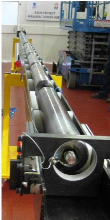
Figure 5 – Super-articulated control rods and seismically qualified nitrogen system at Hinkley Point B reactors
