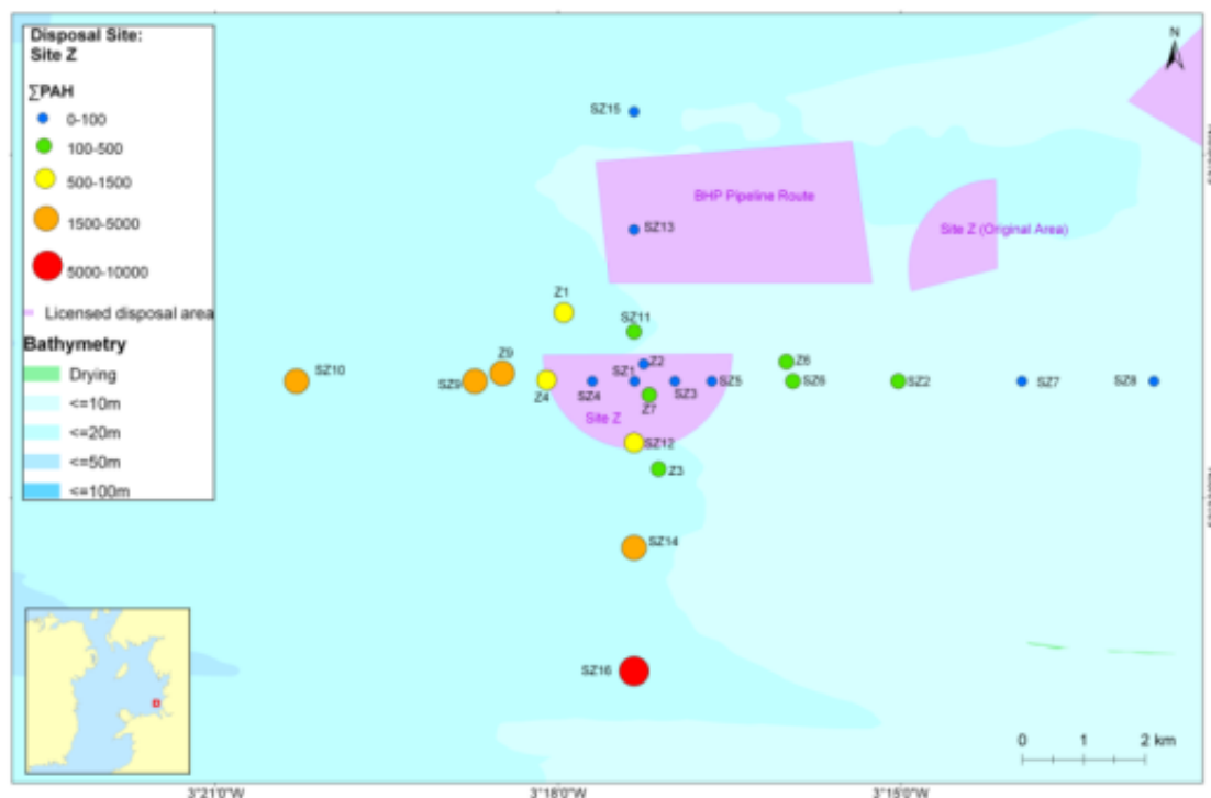
Figure A2.8.10. Summed PAH concentrations ( \mu\text{g kg}^{-1} \text{ dw} ) for stations sampled in 2010 around Site Z in Liverpool Bay.
