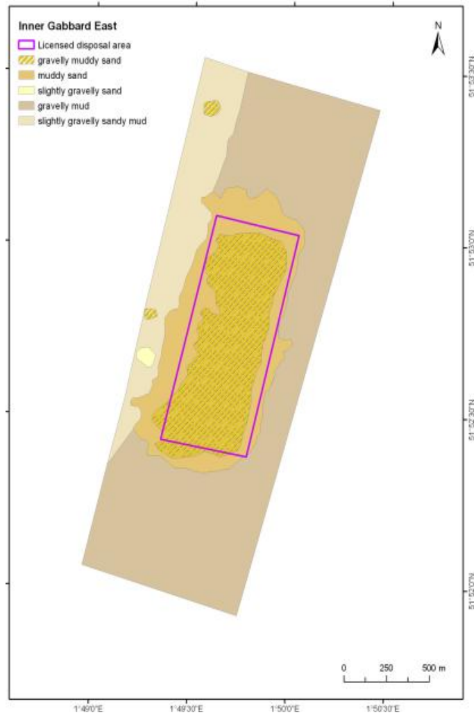
Figure A2.5.5. Interpretation of the multibeam and side scan sonar data collected on the 2010 survey of Inner Gabbard East
