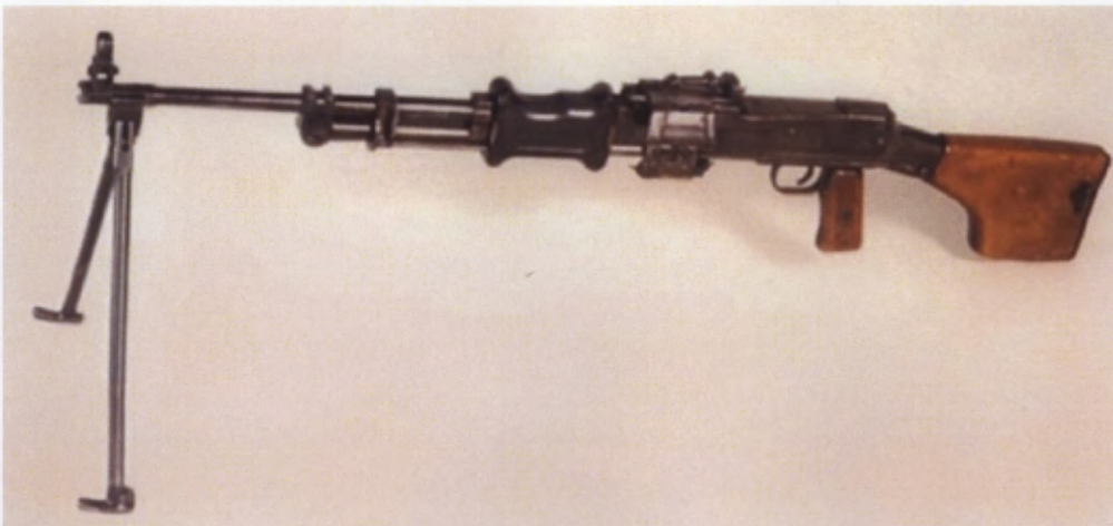
Figure 1-3: RPD belt fed LMG. The belt may or may not be contained in an ammunition box clipped to the weapon in a manner similar to the Minimi. (U)
