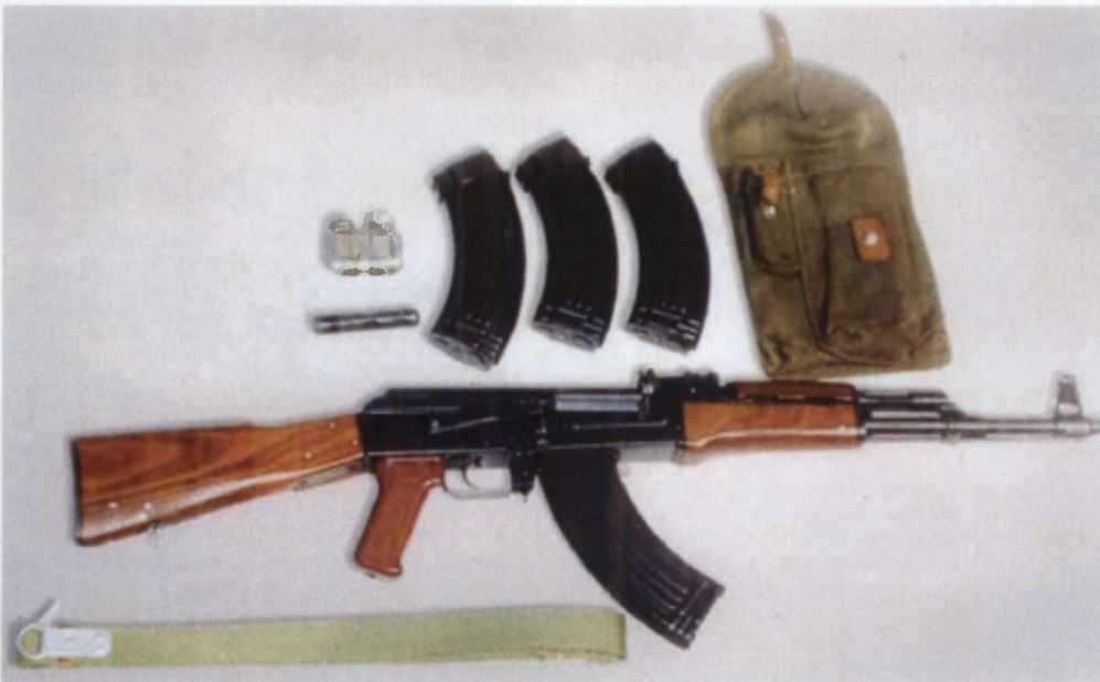
Figure 1-1: Standard AK-47 with accessories. Common variations include a metal or folding stock, shortened weapon, under-barrel grenade launcher, folding bayonet and forward pistol grip, none of which affect the basic mechanism. (U)
