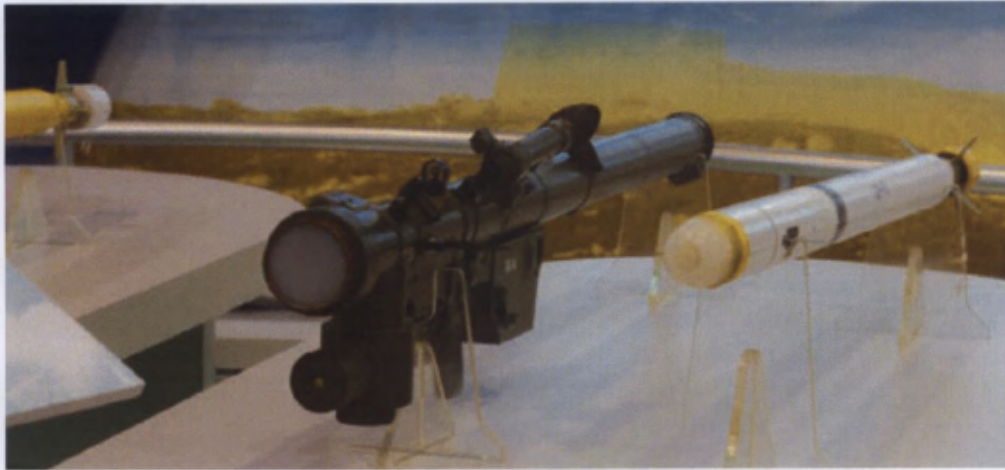
Figure 8-9: A CSA-11 (QW-18) missile and tube with gripstock and battery unit fitted (U)
