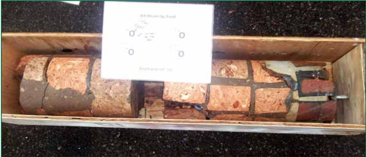
Figure 15: Core taken from tunnel lining during investigation, showing engineering brickwork (right). Core split into two sections during removal (photograph courtesy of Network Rail).
