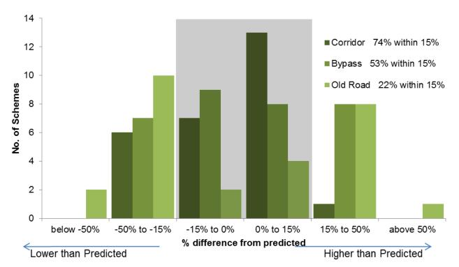
Figure 4–4 Accuracy of Traffic Forecasts (Bypass schemes)
