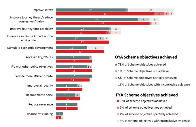
Figure 3-2 shows that a greater proportion of scheme objectives have been achieved at the five year stage, with fewer objectives having inconclusive evidence. The principal reason is due to safety benefits being realised at the five year after opening stage, when at the one year after opening stage the impact was inconclusive (usually do a shortage of sufficient post opening collision data).
