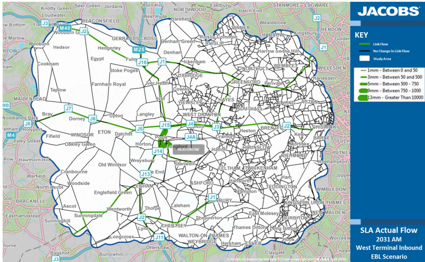
Figure 73: SLA routing of traffic traveling To Heathrow West Terminal Extended Baseline AM On the strategic road network surrounding Heathrow
