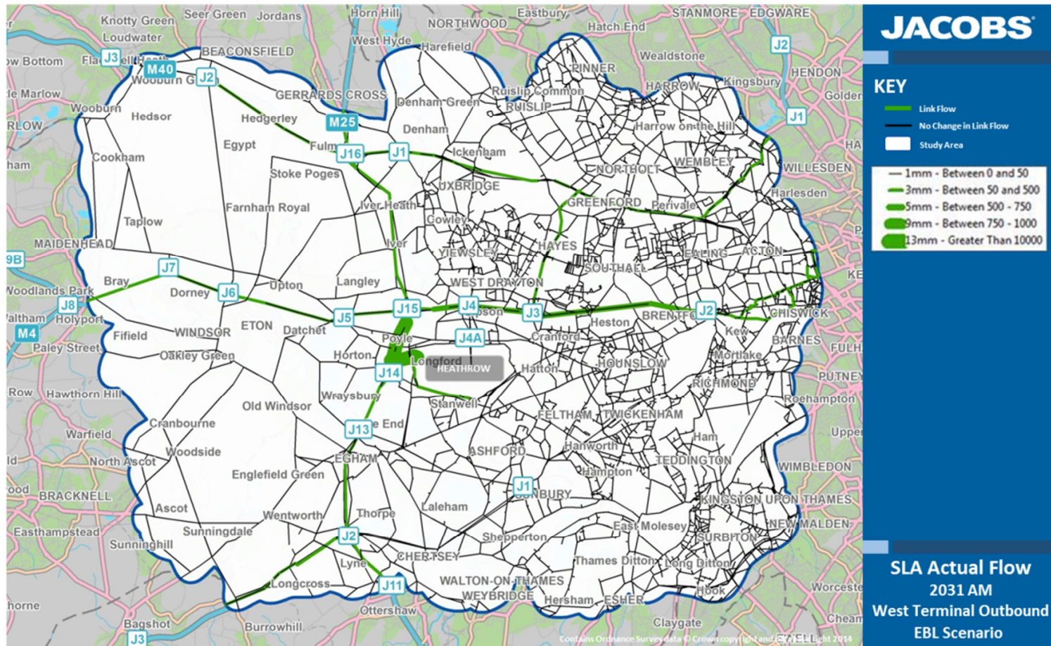
Figure 82: SLA routing of traffic traveling From Heathrow West Terminal Extended Baseline AM On the strategic road network surrounding Heathrow
