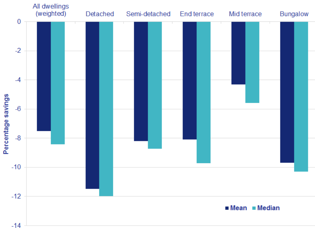
Figure 4.1: Observed savings (weighted) in gas consumption for three bedroomed properties having cavity wall insulation installed in 2013, by property type
