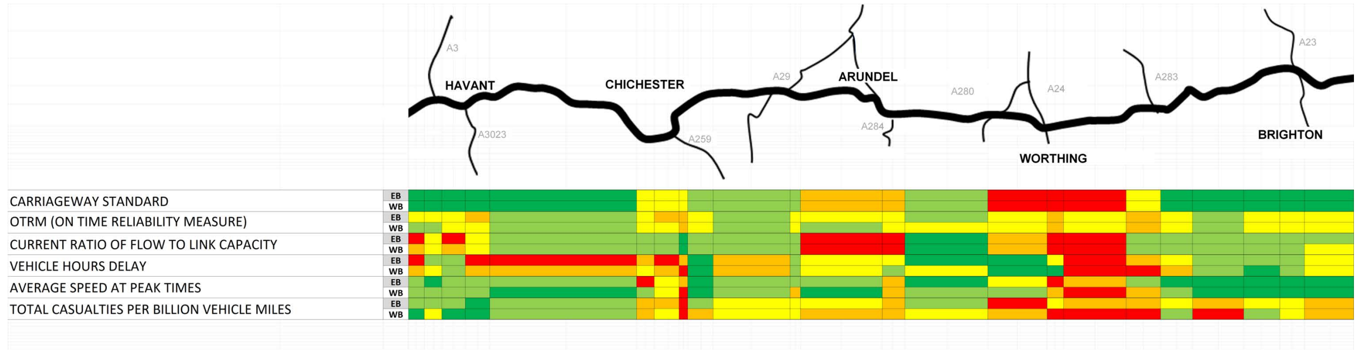
Figure 4-5: Summary of Current Travel Conditions along the A27
