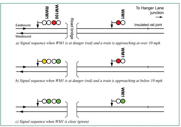
Figure 4: Signal sequence for an eastbound District Line train approaching Hanger Lane junction
