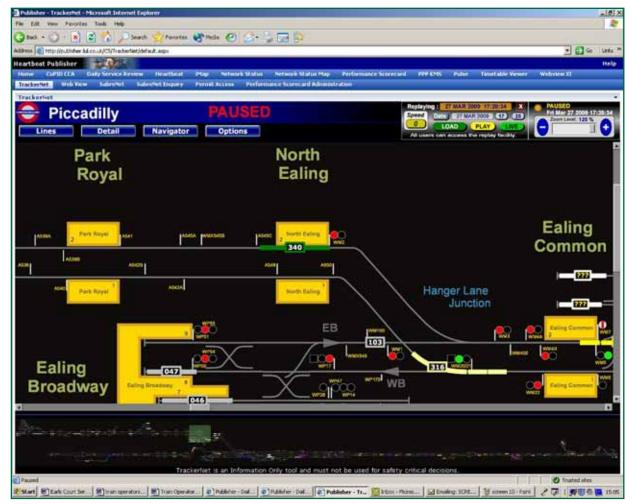
Figure 11: Trackernet screen image at 17:28:34 hrs showing train 316 crossing junction ahead of train 103
