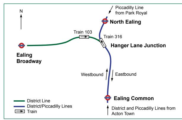
Figure 2: Simplified map of Hanger Lane junction showing position of trains during incident
