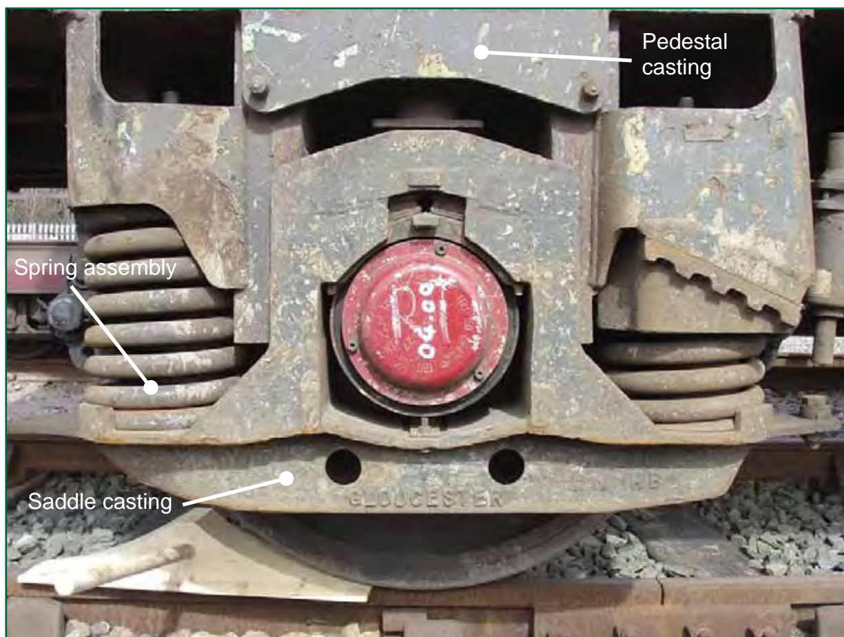
Figure 5: SSA pedestal suspension as fitted to wagon 470152
