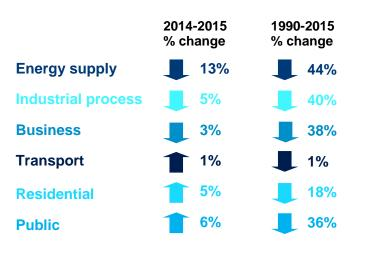
Reduction in energy supply CO<sub>2</sub> emissions driven by change in fuel mix for electricity generation in 2015, with less use of coal and more use of nuclear and renewables
