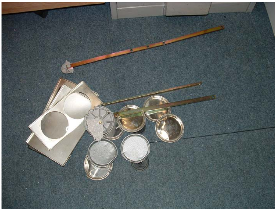
Figure 3: Debris ejected from GPR enclosure including interconnecting bar.
