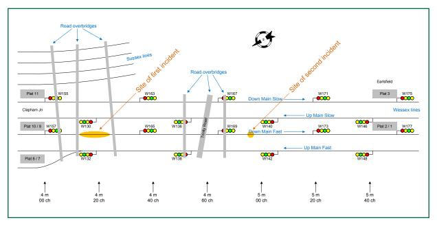
Figure 4: Track layout showing the Wessex lines between Clapham Junction & Earlsfield
