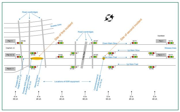
Figure 5b: Layout of the ESR equipment installed on the Down Main Fast line on 8 March 2011
