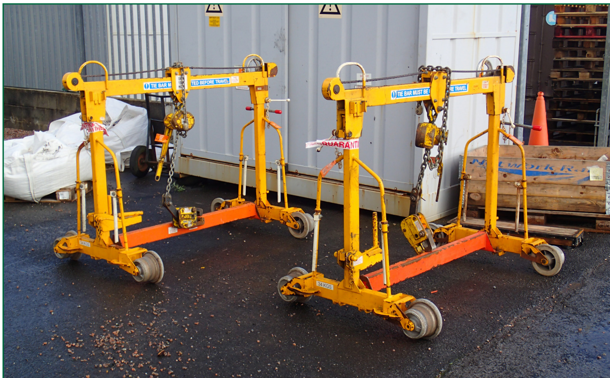
Figure 7: The runaway ironmen after the incident
