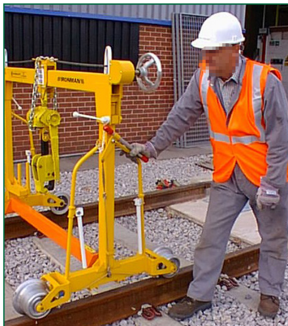
Figure 6: Use of brake handle to release ironman brakes (courtesy Permaquip)
