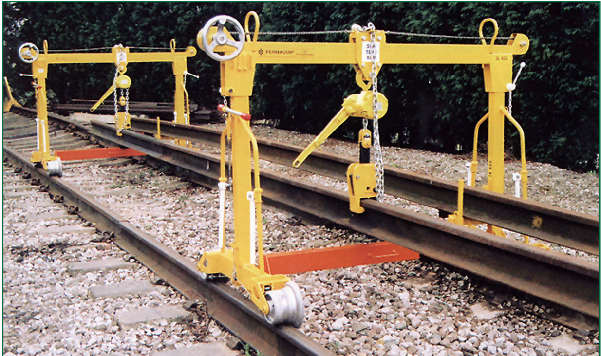
Figure 2: View of a pair of ironmen carrying two lengths of rail (courtesy Permaquip)
