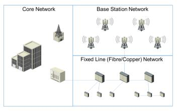
Figure 15: Simplified Private Radio/Fixed network architecture
