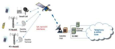
support for fronthaul/backhaul caching. Figure 38: Use of satellite in cellular networks
