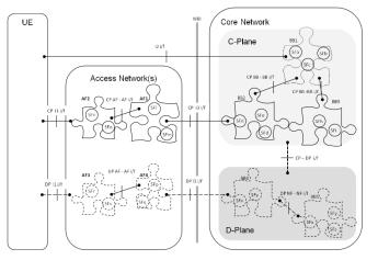
Figure 35: Template for 5G infrastructure architecture<sup>80</sup>
