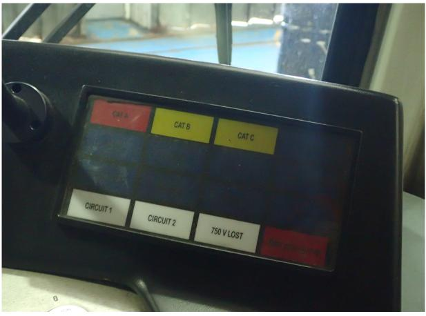
Figure 13: The cab annunciator panel
