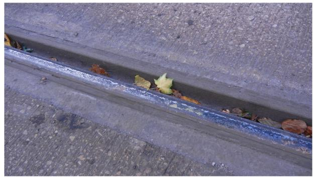
Figure 11: Photograph of rail head at Shalesmoor, taken immediately after accident. Note that rail head is black in colour and the presence of fallen leaves
