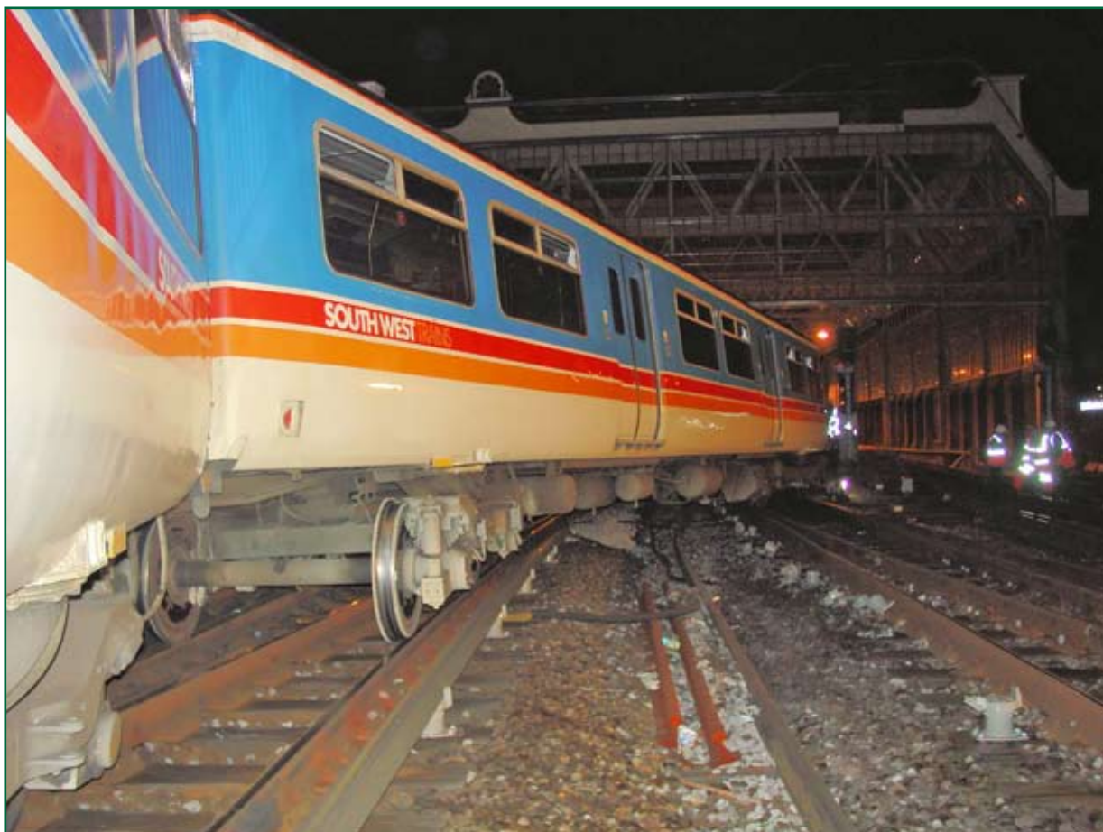
Figure 15: View of rear two carriages of train 1D54 in direction of travel following derailment
