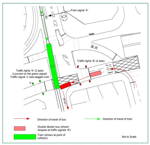
Figure 1: Diagram of road junction showing positions of the tram and bus and the relevant traffic lights
