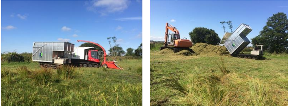
Figure 6: Harvesting activities with PistenBully. Material was being collected by a tracked vehicle, which was taken to a dumped point. The 360 excavator would then pick the material and transfer it to a trailer pulled by a tractor. This area was located close to the entrance.
