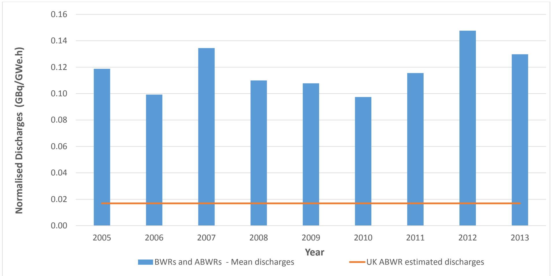
Figure 1. UK ABWR aqueous tritium normalised discharges compared to mean aqueous tritium normalised discharges (GBq/GWe.h) from similar plants worldwide (BWRs and ABWRs) 2005 to 2013
