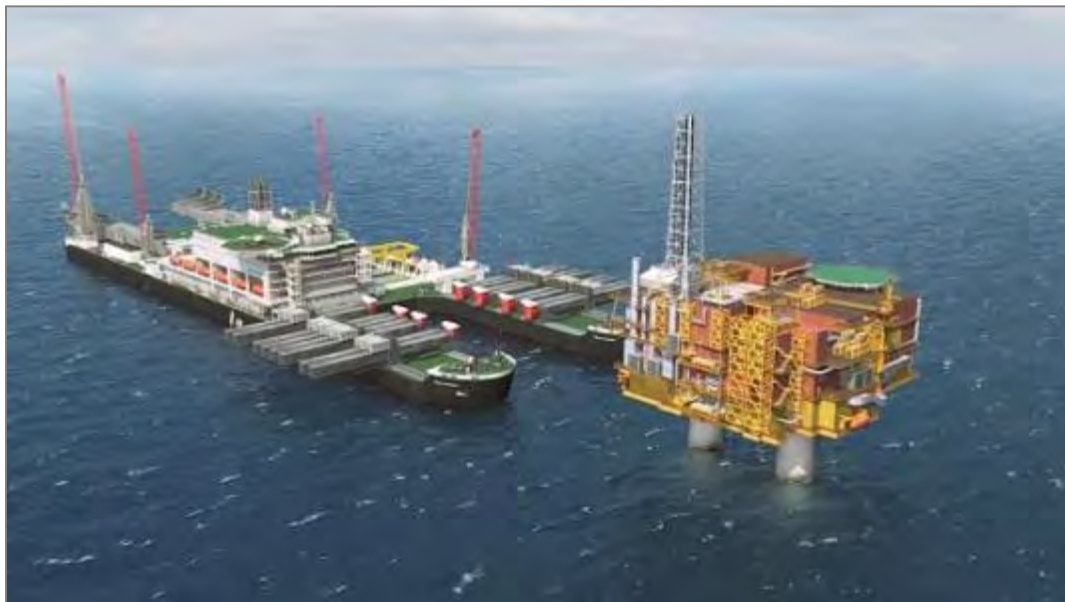
Figure 8-6: SLV Aligning with a GBS
