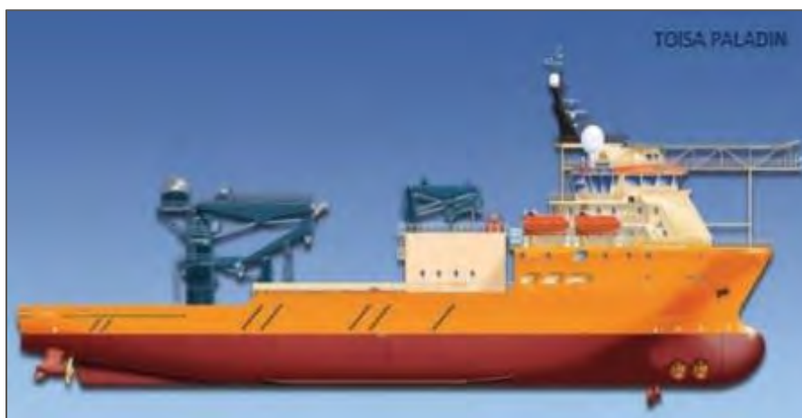
Figure 9-4: Diving Support Vessel (DSV)
