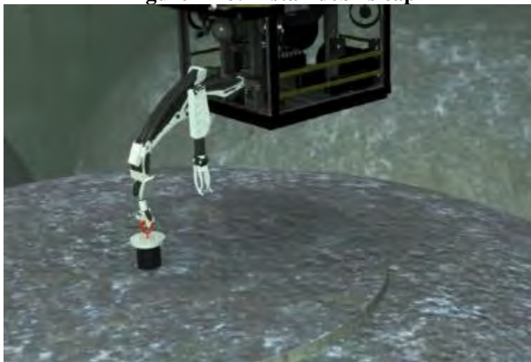
Figure 11-8: Install debris cap
