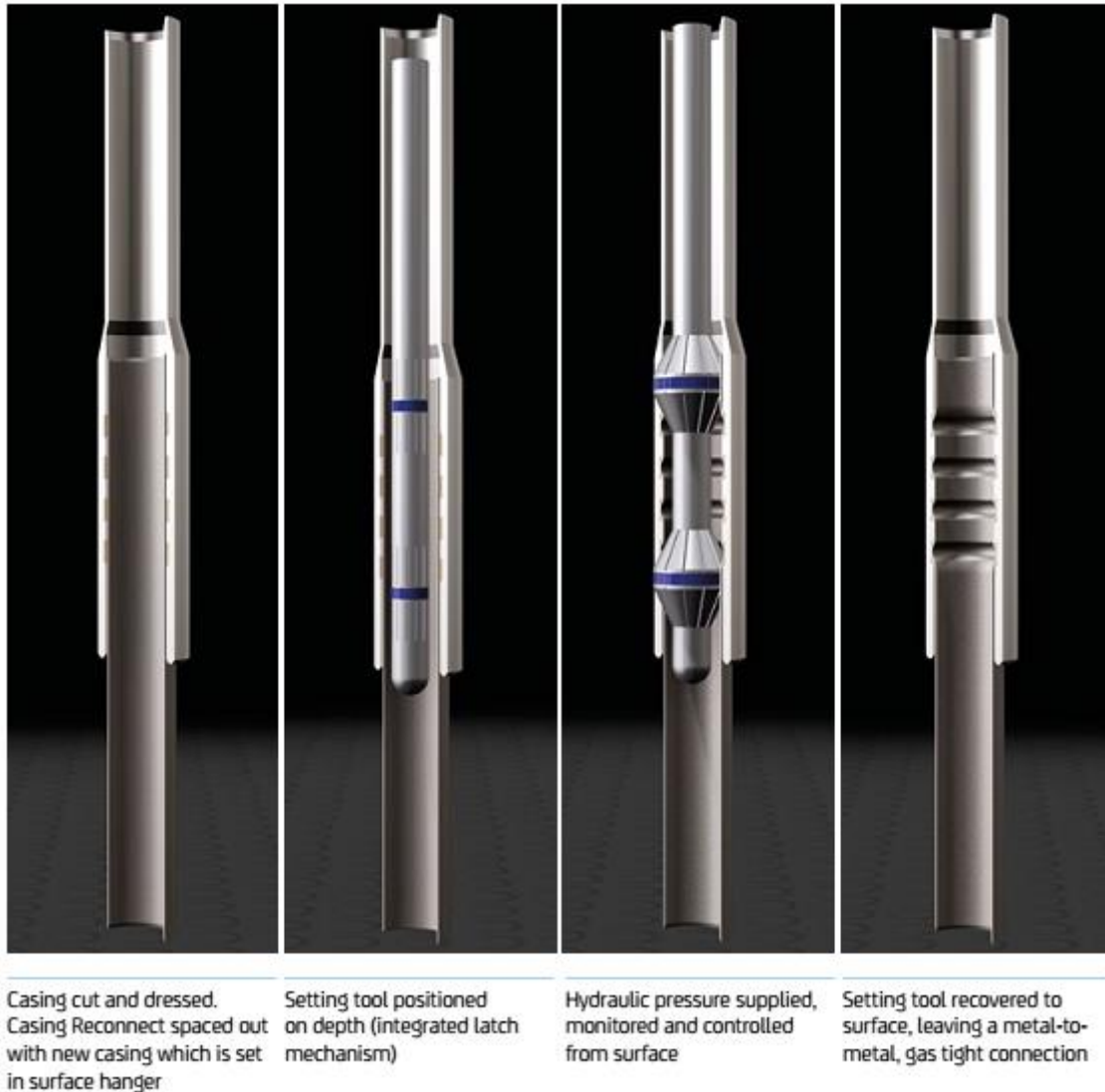
Figure 5.7: Casing Re-connect Operational Sequence
