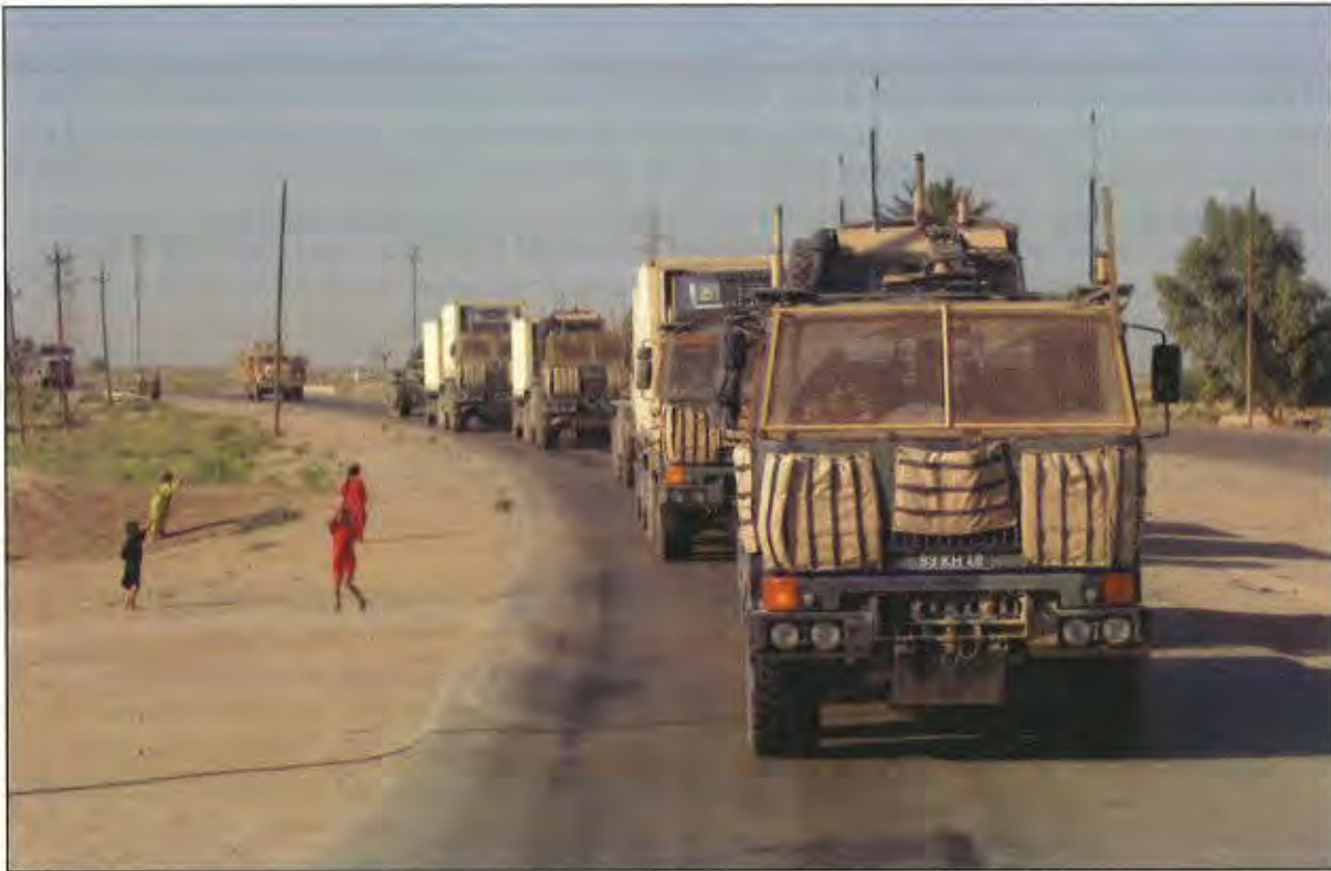
Fig 49. Logistics convoy moving south on the MSR towards Kuwait. Note the Webley Scott improvised armour on the vehicles and the Mastiff and Warrior force protection element.
