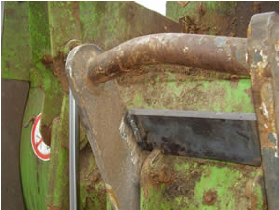
Figure 4 showing lift hook modified to reduce risk of false engagement
