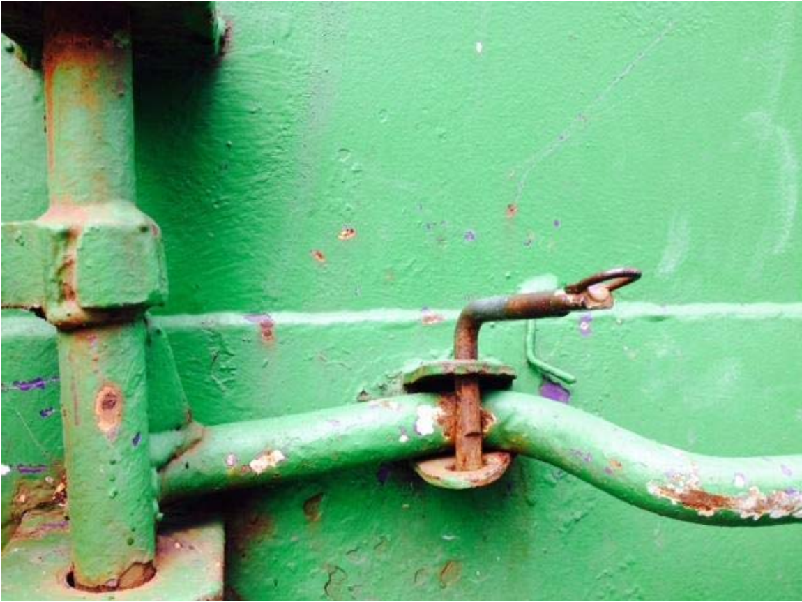
Figure 3 showing light duty mechanism with partly engaged safety pin
