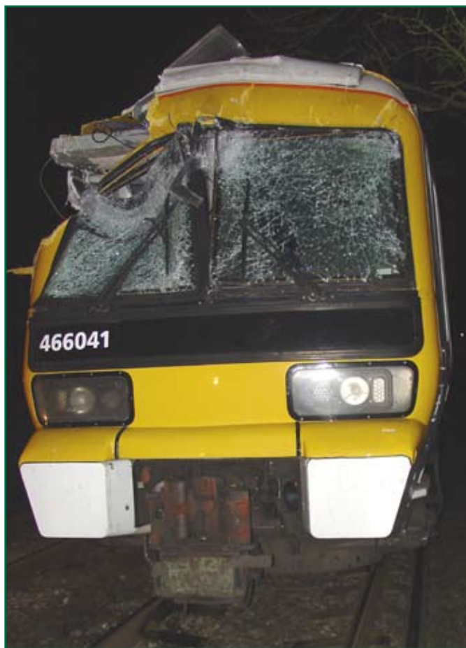
Figure 2: Leading carriage 78352 of unit 466041 showing the external damage sustained
