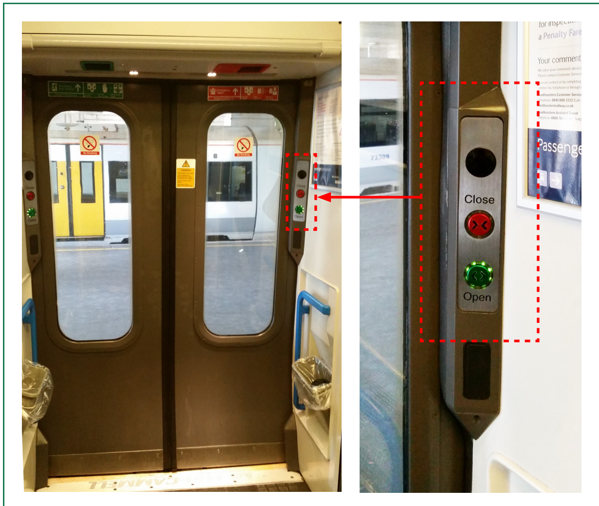
Figure 5: Passenger bi-parting doors and passenger door-open push-buttons
