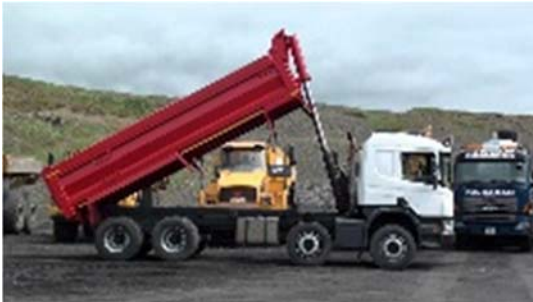
Excavated, demolition materials (32t rigid HGV)
