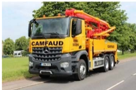
Concrete pump (rigid HGV)
