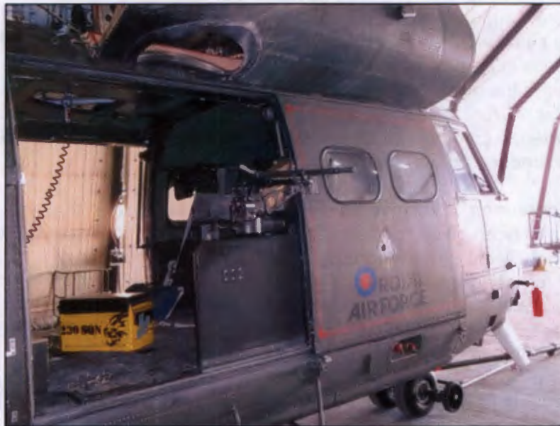
Figure 1.4.3 Image showing restricted access to passenger Cabin caused by Crew Served Weapon
