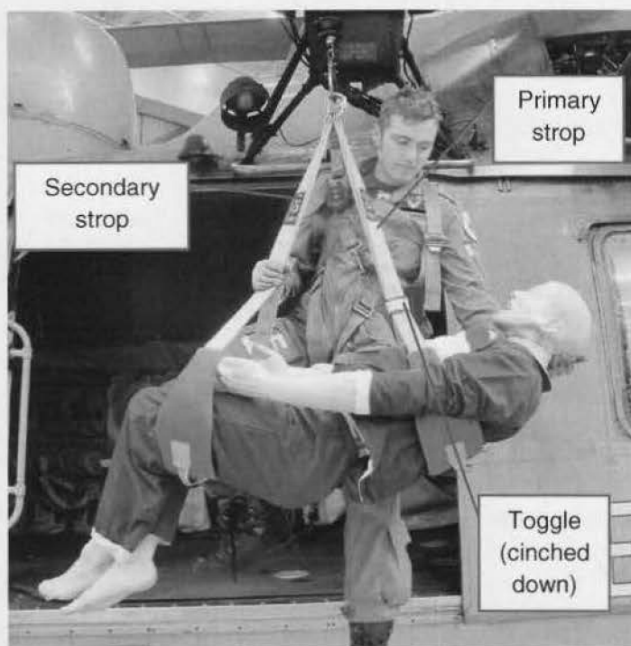
Figure 2 – Dummy in double lift with 2 strops
