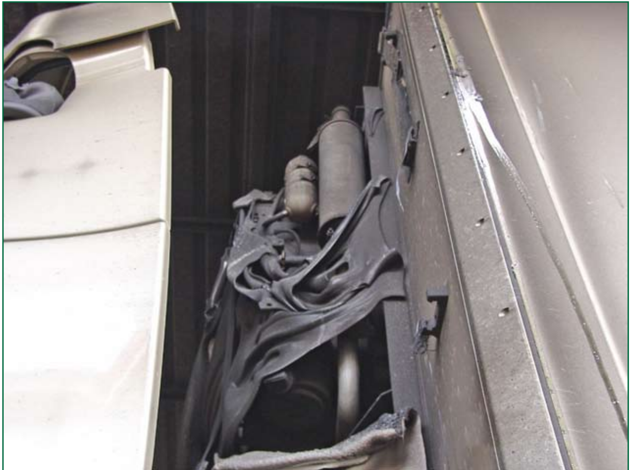
Figure 5: Damage to refrigeration unit of HGV behind incident wagon
