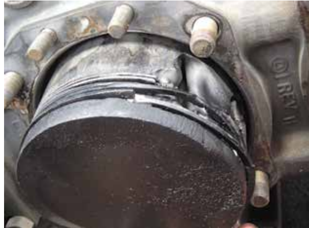
Figure 3 Damaged No 3 piston on right-hand engine
