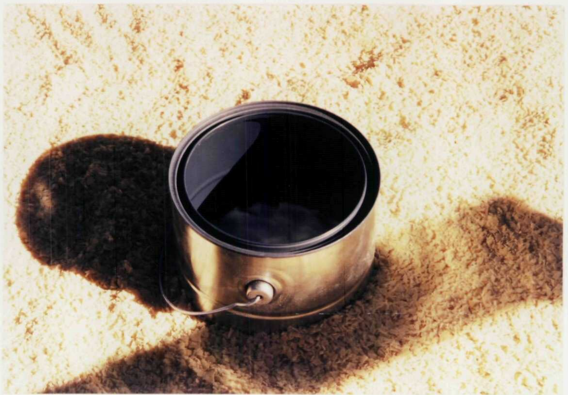
Figure 10. 1000 kg flake TNT charge showing C4 booster
