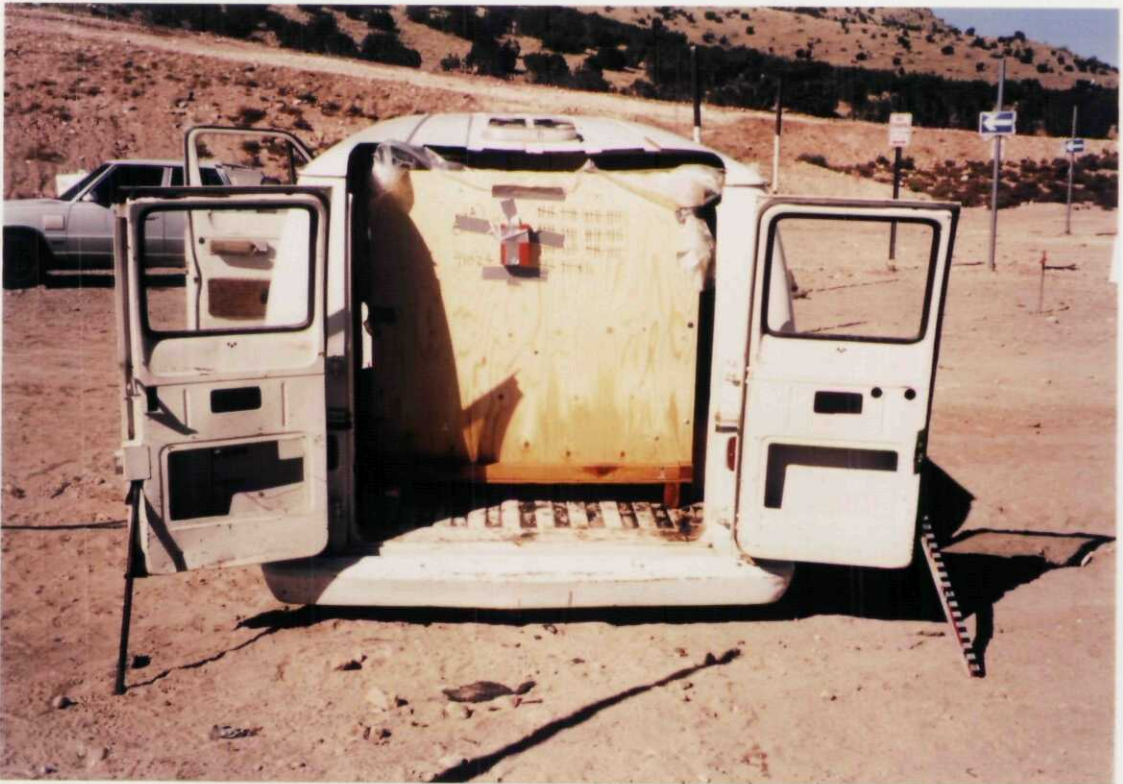
Figure 9. 1000 kg ANFO charge showing position of wooden box in cargo hold of van
