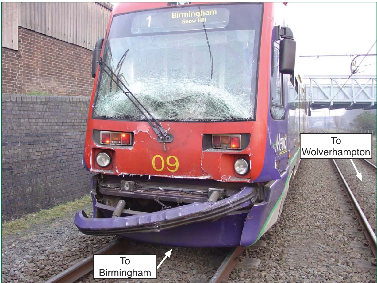
Figure 8: Tram 09 damage to cab
