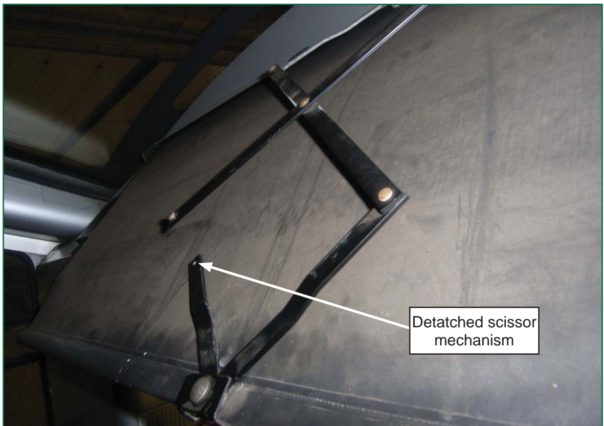
Figure 13: Sunblind mechanism - type I - not capable of operation
