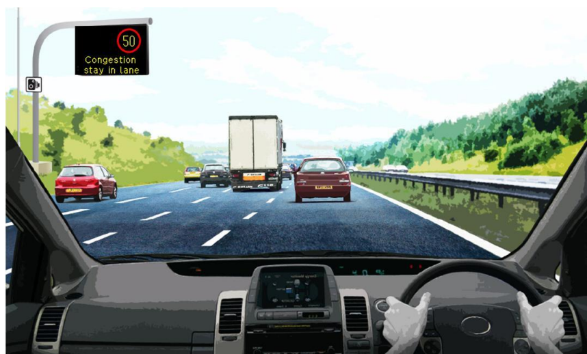
Figure 4D: Illustrative M6 Junction 16 to 19 Smart Motorway All Lane Running scheme section operating with variable mandatory speed limits and information for road users.
