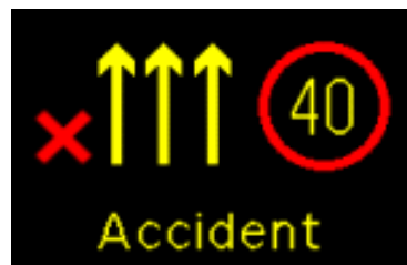
Figure 4G: Variable message sign warning of a closed lane ahead due to an accident
