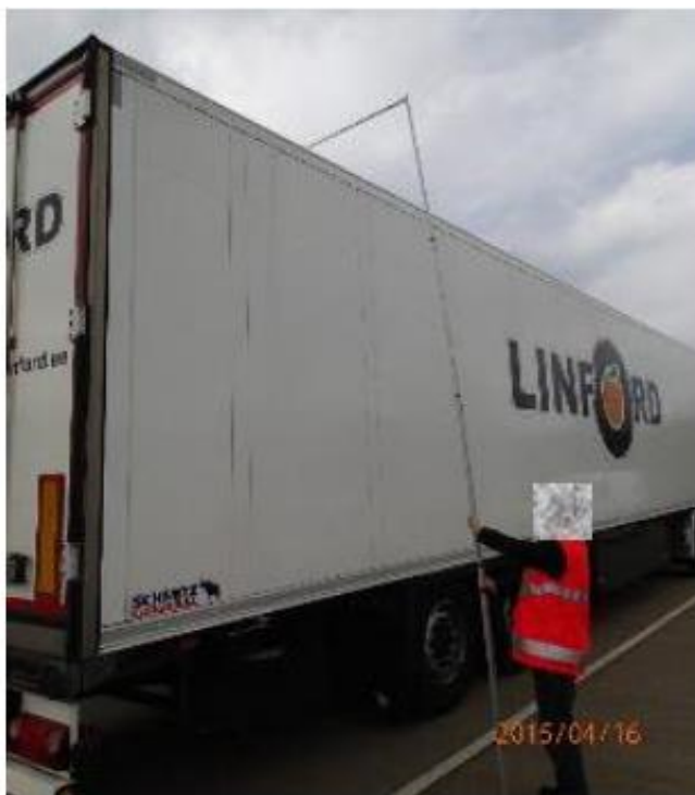
Figure 22: Physical height measurement at the Freight Driver Information Centre
