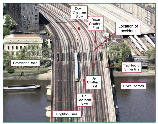
Figure 2: Aerial view, looking north towards Victoria station, of the railway lines crossing Grosvenor Road Bridge, showing the normal direction of rail traffic. © Metropolitan Police
