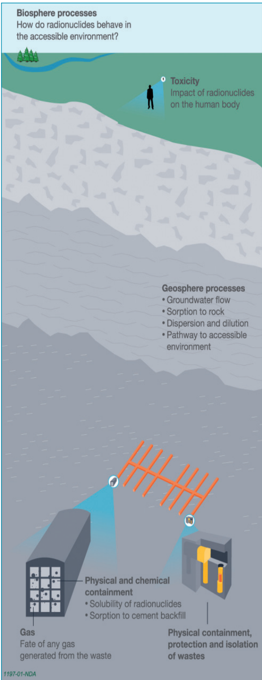
Schematic of the main processes in our geological disposal facility system model
