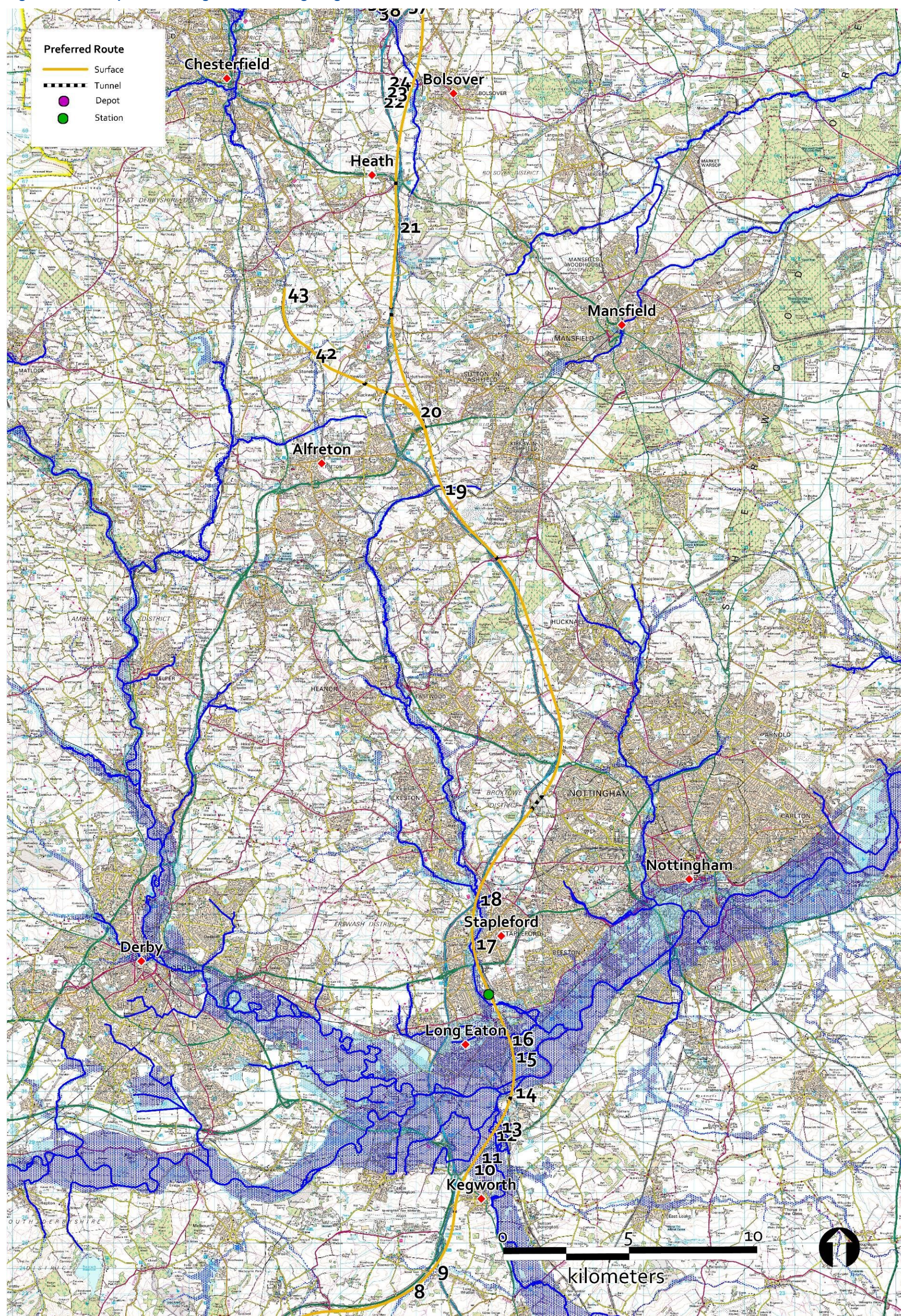
Figure 10-8 Floodplain Crossings – Eastern Leg: Kegworth to Heath
