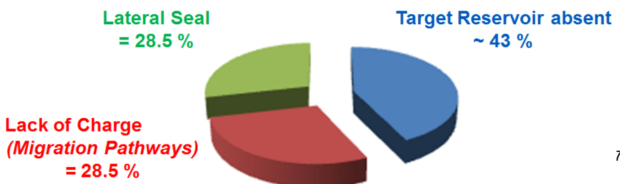
Fig. 202 - Fulmar interpod main reasons for failure
