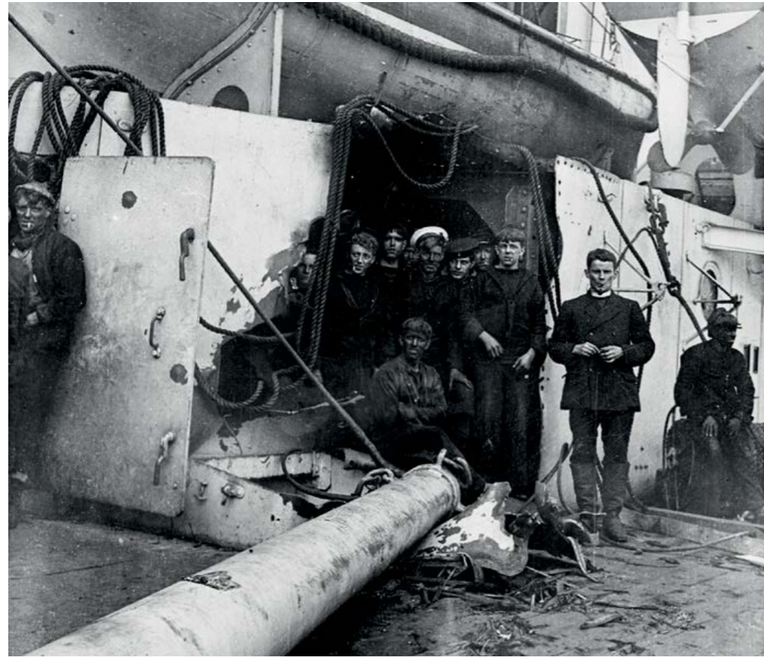
A shell hole on the shelter deck of HMS Tiger © IWM SP1604
