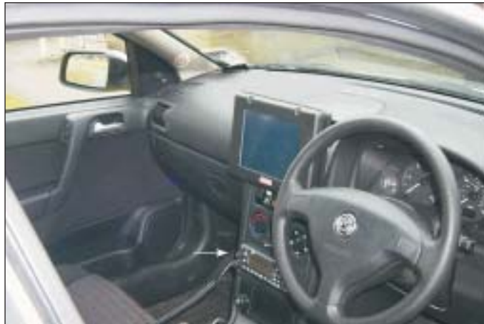
FIGURE 5 Police car interior showing parts of the TETRA vehicle-mounted terminal
