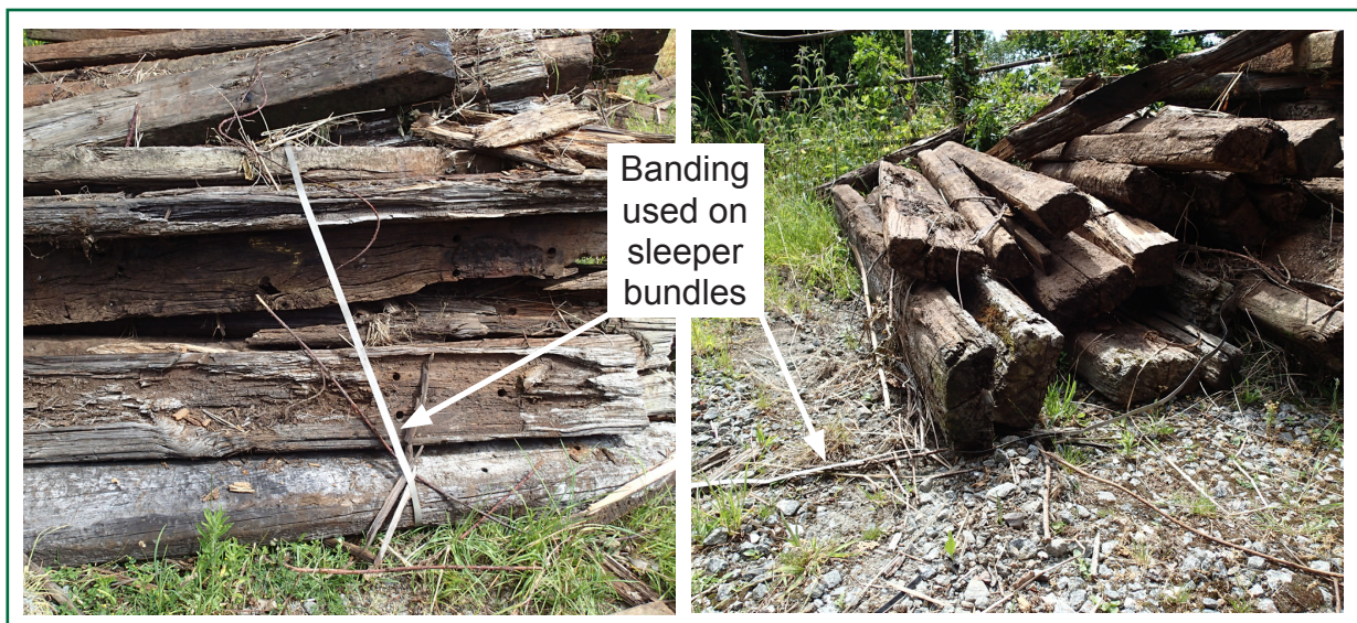
Figure 6: Broken banding around the sleeper bundles
