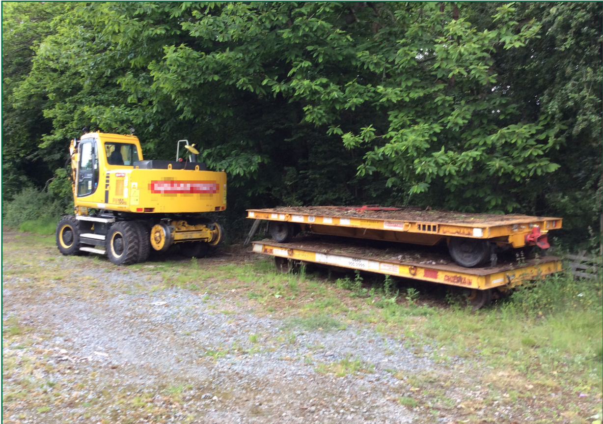
Figure 5: The RRV and trailers (image courtesy of Network Rail)
