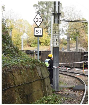
Figure 3: Speed restriction sign. The legend 'SI' under the speed figure indicates the location of a section isolator, an insulated joint in the overhead electrical power line
