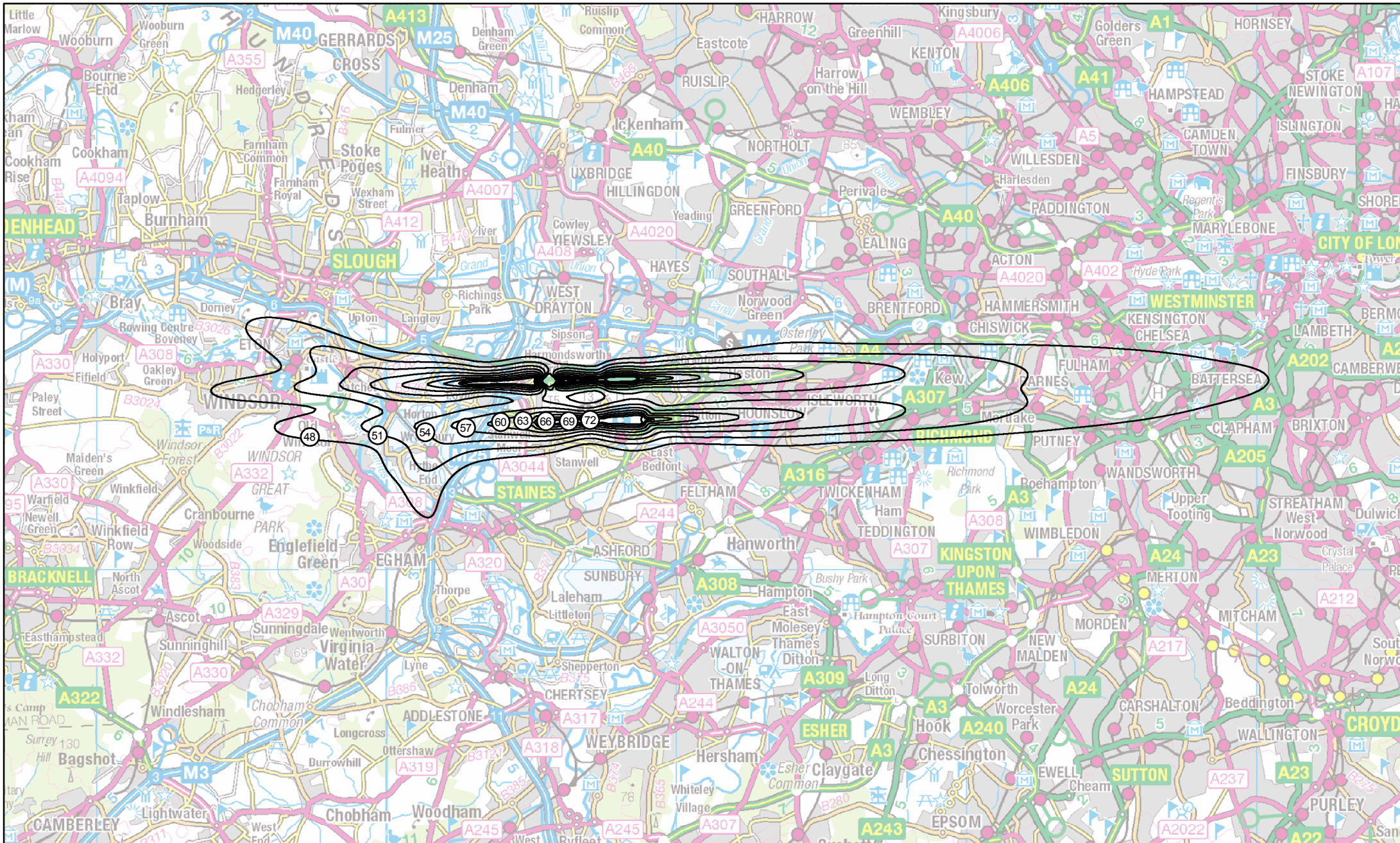
H50-HH-X: Heathrow 2050 do-something, Hub - no sensitivity test Summer average 8-hour night-time LAeq,8h
