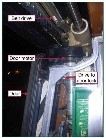
Figure 1: door drive and locking mechanism
