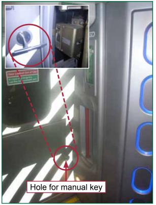
Figure 2: Internal view of door (Inset: Close-up of key in door, and bolt engaged (panel removed to show mechanism))
