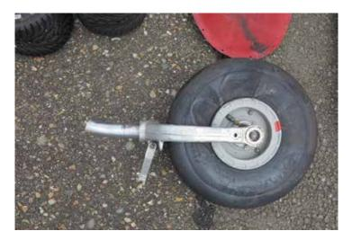
Figure 3 Break in the nose gear jack
