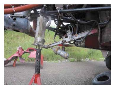
Figure 2 Nose landing gear drag brace
