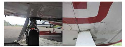
Figure 1 Creasing on the underside of the left wing
