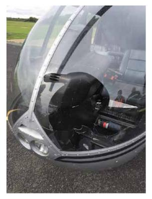
Figure 1 Damage to left windscreen of G-BZGO
